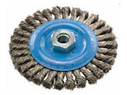
Knot-twisted brushes are for surface cleaning after welding, to remove scale, spatter, rust and corrosion
