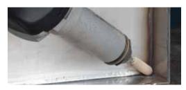
These points are made with high quality BLENDEX U material and offer a fast way to blend, clean and polish in difficult to reach areas. 1/4" shaft
