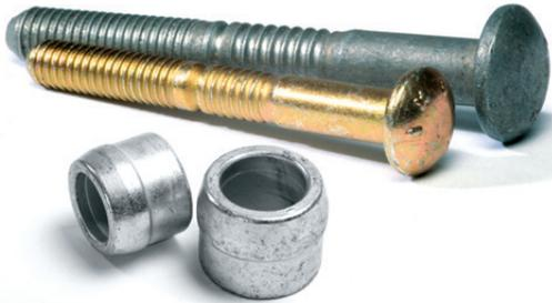
The Huck C6L® is the classic 6-groove locking fastener for a wide range of applications where a strong, vibration-resistant clamp is required. The C6L's exclusive locking groove design ensures a permanent fit that resists loosening, reducing labor and installation costs, along with rework and warranty expenses. The C6L virtually eliminates installation errors, too, because once the collar swage is complete, the pintail breaks off and the fastener is tightly installed.
