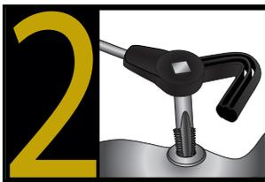
Using the correct size STI (Screw Thread Insert) tap and new 3-way tool, rethread the hole to accommodate the insert.
