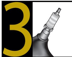
Screw insert in until flush with top of threaded hole. Insertion may be more easily facilitated by using the spark plug where the hole is recessed.
