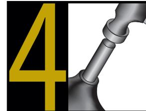
Place expansion tool into insert and hit several times to expand the knurl. Install the spark plug to recommended torque. Do not run engine until sealant has set (refer to manufacturer's specifications).
