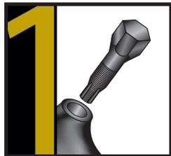
Pack tap with heavy grease. Hand start tap. Then turn with socket wrench to tap hole full depth. Remove chips from hole.
