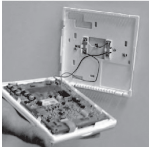
Fig. 10 - Connect Pigtail Wires to Display Module
