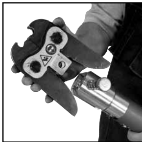
Figure 7: Placement of adapter jaw into the tool
