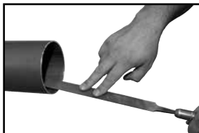
Figure 2: Deburr inside diameter using a half-round file
