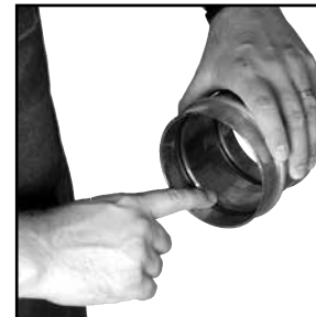
Figure 5: Check for EPDM seal
