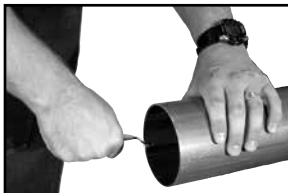
Figure 3: Deburr inside diameter deburring tool
