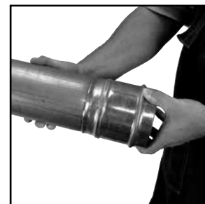
Figure 9: Inspection of final crimp
