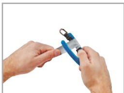
WRAP TAPE AROUND TOOL & TAIL
