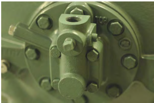
Fig. 19 — OPSS Sensor Block Installed
