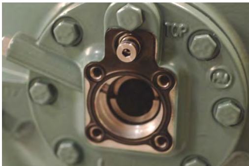
Fig. 18 — OPSS Sensor Block Gasket
