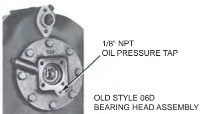
Fig. 8 — 06D 2-Cylinder Compressor Connection Points
