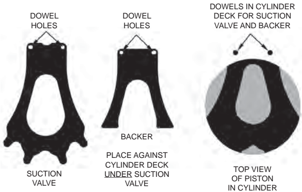
Fig. 5 — Piston, Suction Valve, and Backer Positions (06E)
