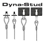
**Step 1:** Insert and tighten the Dyna-Stud into a threaded receptacle of the corresponding size. A locking jam nut is recommended to prevent the Dyna-Stud from turning. \*If using Drop-In see instructions below.
