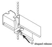
**STEP 4:** To adjust the cable lock, take the load off and pull the wire rope tail slightly to disengage the cable lock teeth. Then release the wire rope by pulling on the "T" shaped release.
