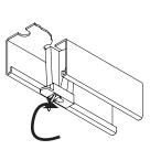
**STEP 2:** Insert the cable lock into the strut.
