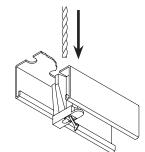
**STEP 3:** Pass the wire rope through the hole in the strut and into the cable lock until at least 6" of wire rope exits the cable lock.
