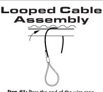
**Step #1:** Pass the end of the wire rope around the anchor point and through the cable loop.
