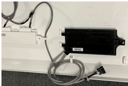
Fig. 24 — Front Panel with New Display Board and Adapter Board
