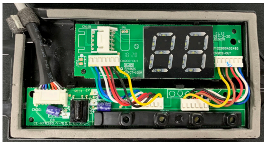
Fig. 19 — Display Board Installed on the Display Board Holder
