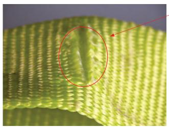
THE DAMAGE: **Holes/Snags/Pulls**WHAT TO LOOK FOR: **Punctures or areas**where fibers stand out from the rest of the sling surface.
