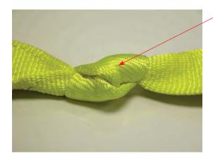
THE DAMAGE: **Broken/Worn Stitching** in the main stitch patterns of web slings has a direct adverse effect on the strength of a sling. The stitch patterns in web slings have been engineered to produce the most strength out of the webbing. If the stitching is not fully intact, the strength of the sling may be affected.
