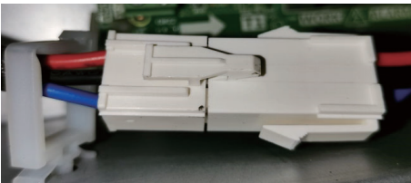
Fig. 28 — Insert the white plug wire
