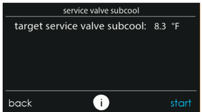
Fig. 13 – Liquid Service Valve Subcooling Target
