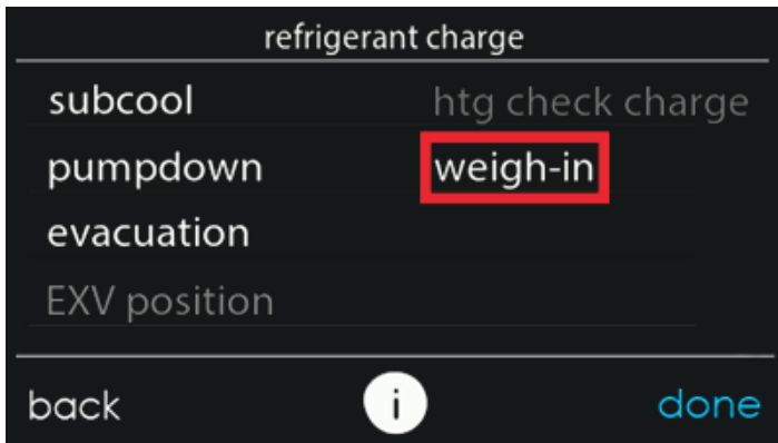
Fig. 15 – Weigh-in Option for charging below 65°F OAT and above 105°F OAT A200034
