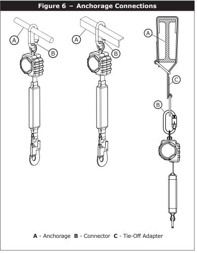
Connect the Swivel Eye (Rebel components identified in Figure 2) to the D-Ring on the harness using the Carabiner included with some Rebel models (or use a suitably rated connector), or use the included Snap Hook to connect to the D-Ring. The opposite end of the Rebel must be connected to an anchorage point (see Section 2.3) with an included Carabiner (or a suitably rated connector), or the included Snap Hook.
